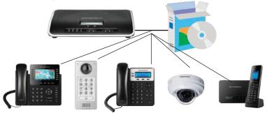
Our UCM series offers Computer Telephony Integration (CTI) which allows you to share all of its features and functionalities with third party software, such as billing software. This allows our UCM to be synced with, for example, a restuarants' customer service software, to support features like calling customers when their table is ready.
