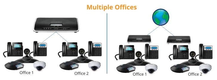
For business with multiple locations, multiple UCMs can be peered together, or a centralized UCM can support multiple locations. Peering allows all employees to be on the same network no matter what office they are in, while also making installation and management as simple as possible.
